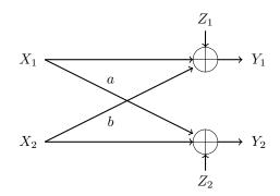
Fig. 5: Gaussian interference channel
