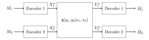
Fig. 1: Discrete memoryless interference channel
