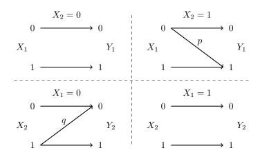
Fig. 2: Binary skewed-Z interference channel (BSZIC)
