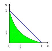
Fig. 3: Regime of parameters where sum-rate capacity is established for very weak BSZIC(p,q)
