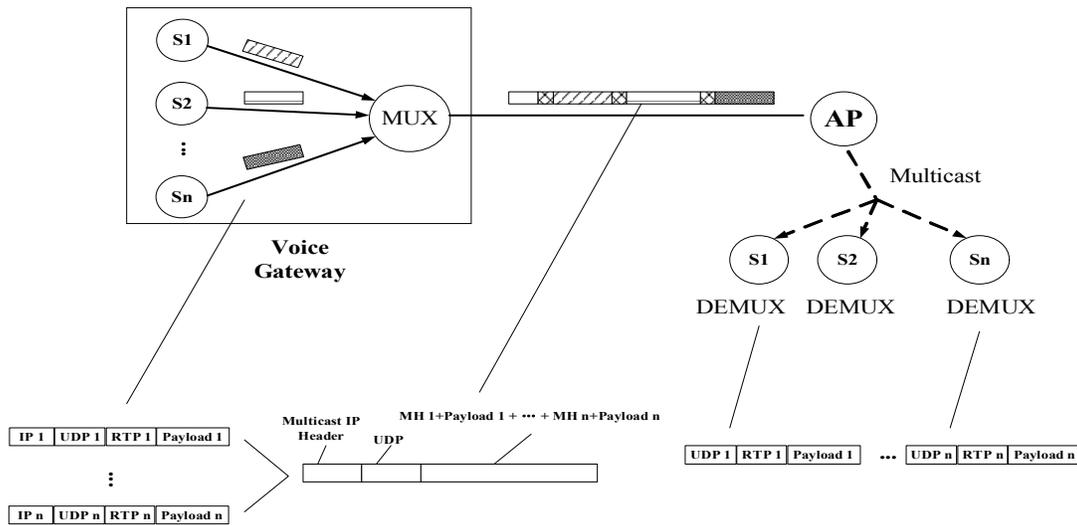
**Figure 3. MUX/DEMUX Procedure**
