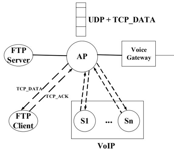
**Figure 8. Setup for Experimental Studies of VoIP-TCP Interference**
