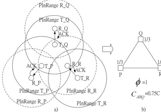
Figure 3. Mapping of a network topology with ARQ a) to b) ARQ physical interference graph
