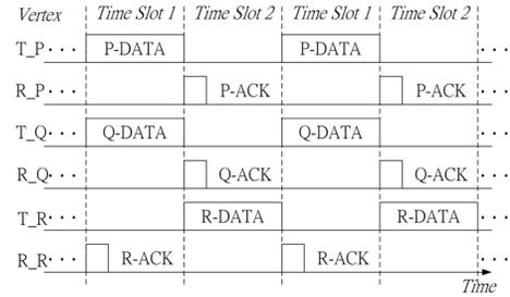
Figure 6. Scheduling the transmissions of links in the network topology of Fig. 3a according to the colouring result of l-graph in Fig. 4b
