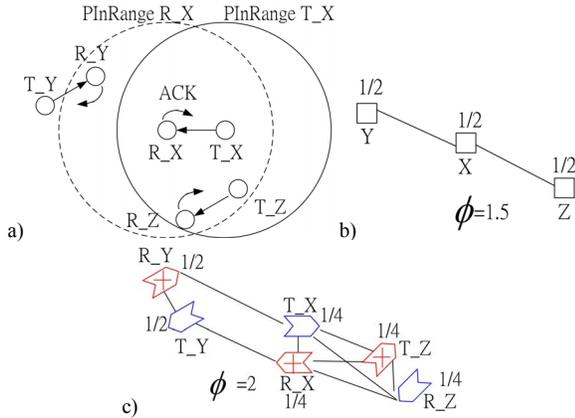
Figure 5. Mapping of a network topology a) to b) ARQ physical interference graph and c) coloured link-directional interference graph
