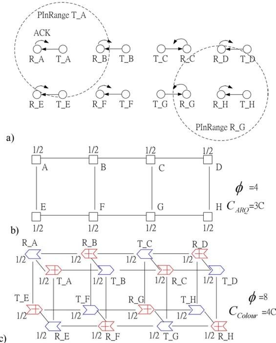
Figure 7. Mapping of a 2x8 lattice topology a) to b) ARQ physical interference graph and c) coloured link-directional interference graph
