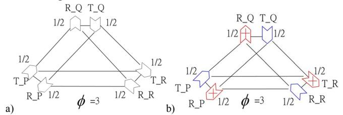
Figure 4. a) Link-directional interference graph of the network topology in Fig. 3b and b) its colouring result
