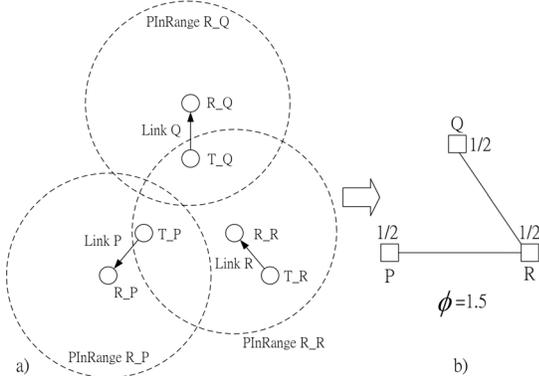
Figure 1. Mapping of a network topology a) to b) physical interference graph
