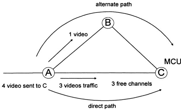
Fig. 3. An example to illustrate the Bifurcated Routing scheme.
