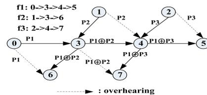
Fig. 1. Illustrative topology for the failure of network coding.
