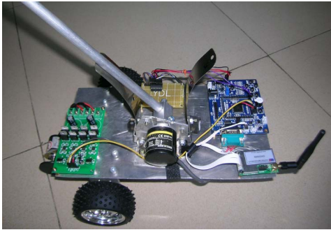
Fig. 2. The pendulum-cart system with the system parameters: M = 1.61\text{kg} , m = 0.09\text{kg} , L = 0.24\text{m} , I = 0.0017\text{kgm}^2 .
