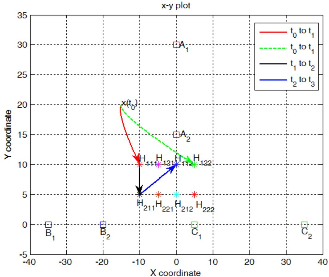
Optimal trajectory of sensor for a three-agent case
